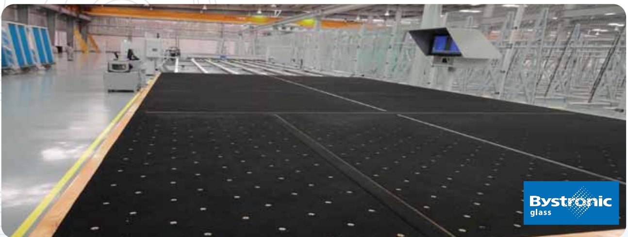
CNC Jumbo Cutting Machine from Bystronic (Switzerland) 3300 X 6100 ( UP TO 19mm) Capacity - 750000 Sqm/year
